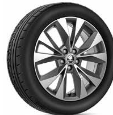
Geneva light-alloy wheel 6.5J x 17" ET40 for 205/55 R17 654 071 497G HA7 | anthracite metallic, brushed
