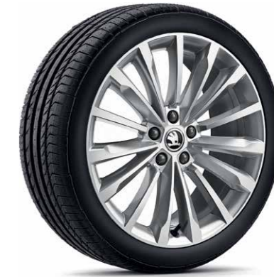
Trinity light-alloy wheel 8.0J × 19" ET44 for 235/40 R19 3V0 071 499E 8Z8 | silver metallic
