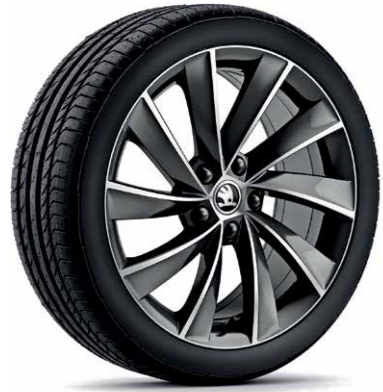
Pegasus light-alloy wheel 8.0J × 18" ET44 for 235/45 R18 3V0 071 498H HA7 | anthracite metallic brushed
