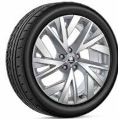
Atria light-alloy wheel 7.5J × 19" ET40 for 235/50 R19 57H 071 499 8Z8 | silver metallic, brushed
