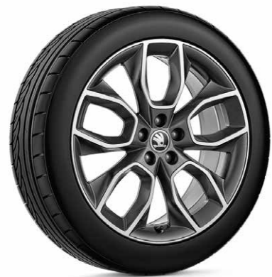
Crater light-alloy wheel 7.0J × 18" ET39 for 215/45 R18 654 071 498N HA7 | anthracite metallic, brushed
