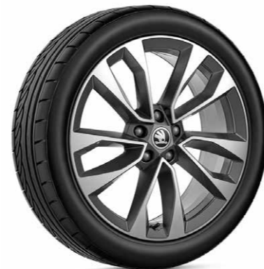
Procyon light-alloy wheel 7.0J x 19" ET43 for 235/50 R19 565 071 499P HA7 | anthracite metallic, brushed
